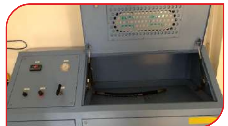
50000 PSI HOSE TESTING CHAMBER.
