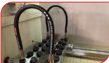
HIGH PRESSURE AND HIGH TEMPERATURE OIL TRANSFER USING 1 SECOND IMPULSES
