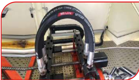
SPIRAL HOSE TESTED FOR 500K CYCLES
