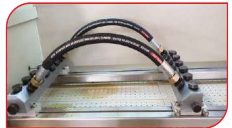
IMPULSE TESTED FOR 200K - 400K CYCLES FOR R1 AND R2
